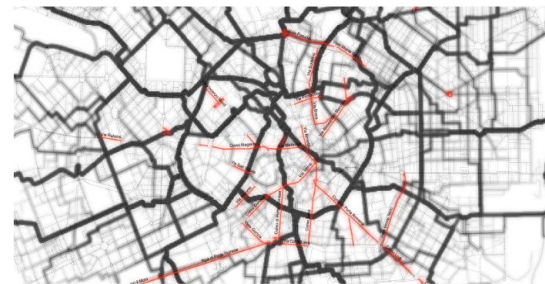
Fig. 4 - Assessment of high impact infrastructural actions. Highlighted in red are high-connectivity roads that are systematically avoided by cyclists due to inadequate conditions.
