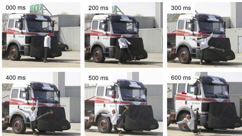
Figure 2: APROSYS nose cone attached to an HGV front end deflecting a pedestrian dummy to the side during an impact test (Feist and Faßbender, 2008)
