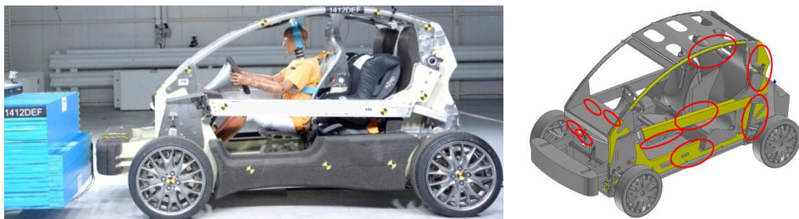
Figure 5: BEHICLE frontal impact test (left) and areas of the BEHICLE fitted with accelerometers (right)
