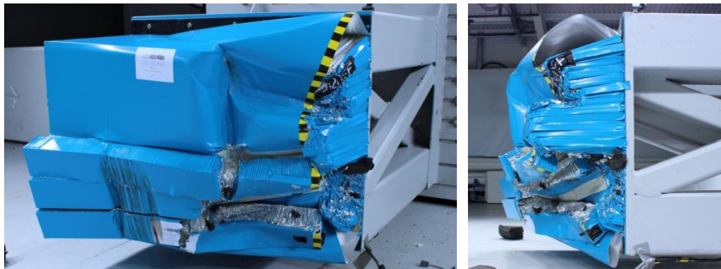
Figure 11: Euro NCAP frontal impact offset deformable barrier post-test
