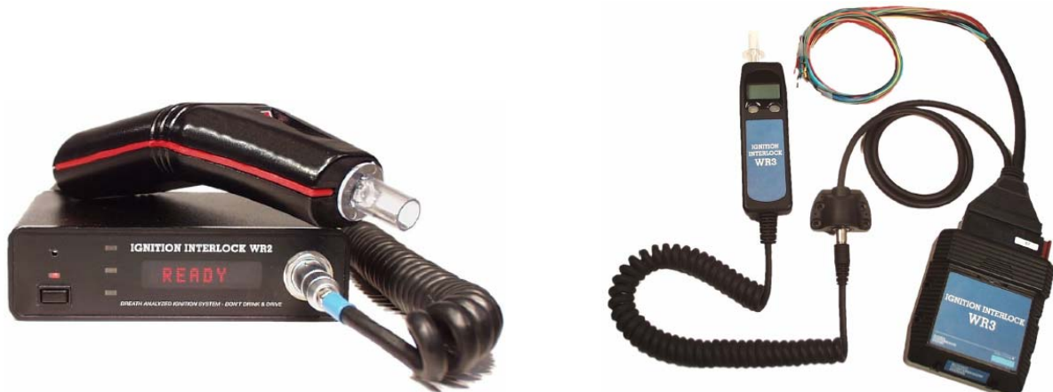
Figure 2: Sample head (left) and control unit of WR2 Interlock (left) and the new WR3 Interlock (right)
